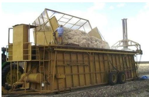
**Picture 17:** Buggy tipping into module maker
